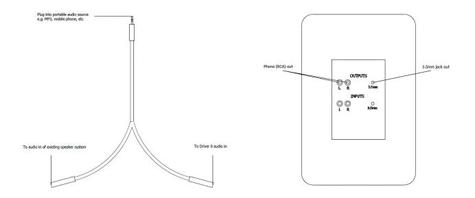
If you use your own personal audio source (mobile phone, tablet, laptop, etc.) into a speaker system for your class, you will need to use the 3.5mm splitter to split the audio signal allowing you to send the audio to both the speaker system, and the Driver 4/8 Pro.
