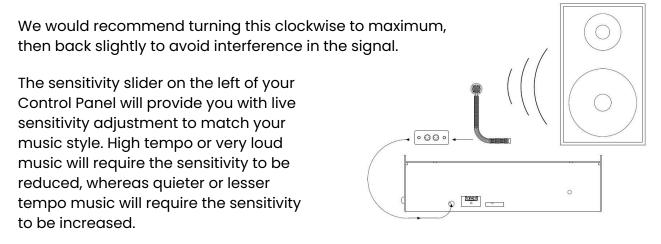
To test the microphone, clap your hands and note if the red LED on the amplifier flashes. If it doesn't you need to press the black button on the amplifier to supply power to the mic.
