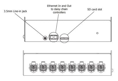
On the base of the Driver 4/8 Pro there are 4/8 LEDSnaps™ PACE outputs. Each output can control up to 20 PACE units, however a maximum of 40/80 PACE bars in total per Driver 4/8 Pro cannot be exceeded.
