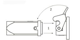
Fully inserted and locked into place
