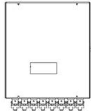
Once you have decided on the ideal location, remove the lid of the driver, there are 4 holes in the rear panel of the driver to affix the driver to a surface such as a wall. Make sure you will be installing the mounting screws into a hard material (wood, brick, concrete), and not a cavity wall. Use suitable screws and plugs to secure the Driver to your surface of choice.
