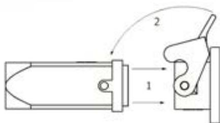
Fully inserted and locked into place
