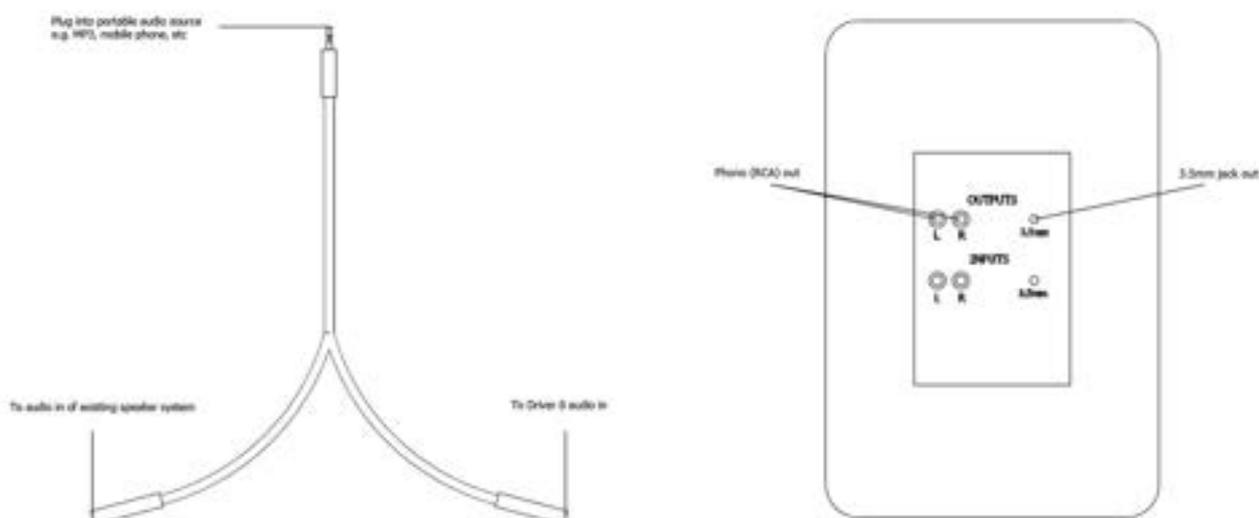
If you use your own personal audio source (mobile phone, tablet, laptop, etc.) into a speaker system for your class, you will need to use the 3.5mm splitter to split the audio signal allowing you to send the audio to both the speaker system, and the Driver 4/8 Pro.
