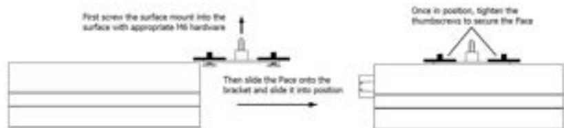
Your first fixing point should be 300mm in from the start of your first LEDSnaps PACE bar, and every 600mm throughout the installation. This will ensure a centred fitting and equal force on each cable.
