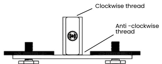
LEDSnaps will not draw any power from your track light so your current power configurations need not change. This is an attachment fitting only. The threaded rod and nut will be pre-fitted to ensure a good fit inside the track light fitting. Simply drop the threaded rod into the fitting and screw it onto the turnbuckle.
