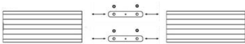
Slide the splicing kits into the two outer channels. Use the holes to locate the correct positions.
